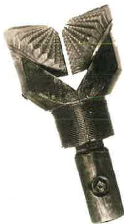
Howard Hughes's rock bit had rotating drills that were able to cut through hard rock.
