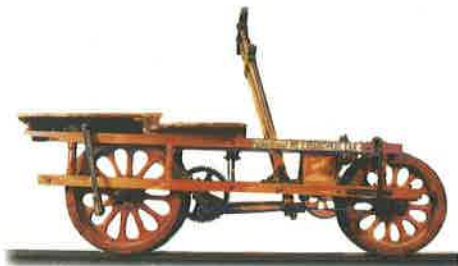
Hand-powered carts were occasionally used as transportation on early rail lines.
